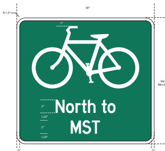
Figure G-2: Conceptual Alternative Bike Route Guide (D11-1c) sign for Croatan Region Bicycle Route
